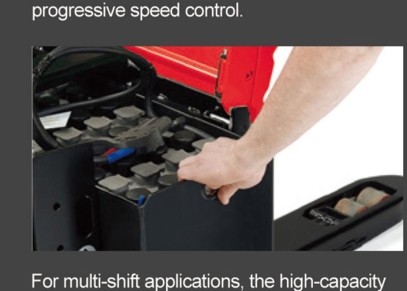
battery is placed on rollers, for quick, easy
