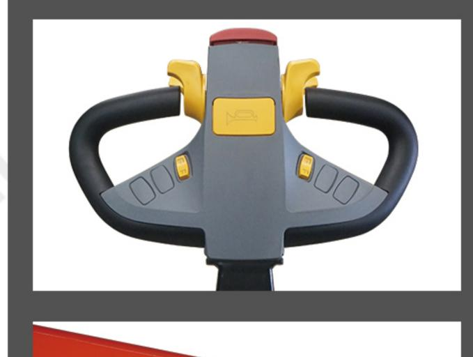
Ergonomic multifunction handle control can beequipped with push button fucntions, emergency safety reversing and large central horn button for safe operation.
