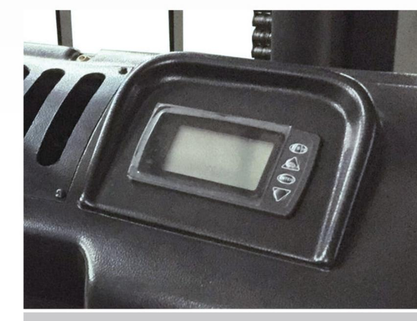
Intelligent programmable LCD display, can show the fault codes, so that the driver and servicer can easily detect machhine's failures, reduce detection time, improve maintenance efficiency.
