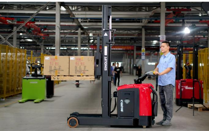
With Max. capacities to 2000kg, the CQXD16/CQXD20 models are built to be the best, most reliable narrow aisle walkie reach trucks in the industry.
